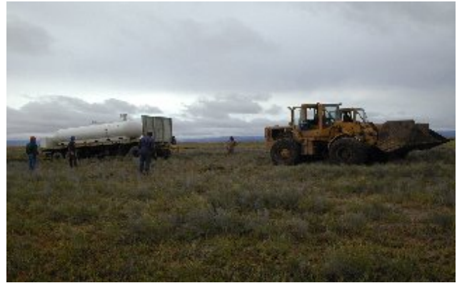
Fig. 3. Hauling of the water transportation trailer with 12 tons of pure water by two caterpillars at a difficult position with wet soil.
