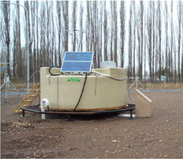
Fig. 4. A WCD deployed at Auger Central Station.
